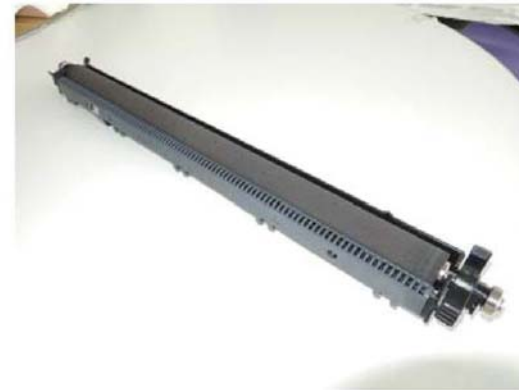
Figure 2 Removed BTR roll
