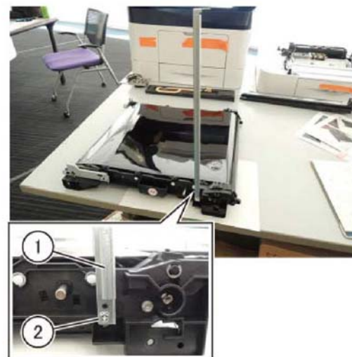
Figure 7 IBT belt unit bottom guide install
