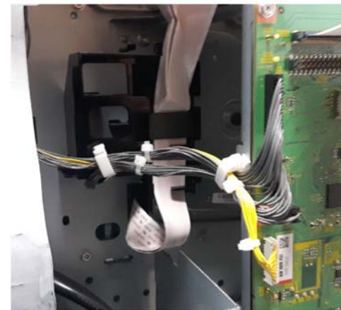
Figure 5 Wire harness removal
