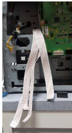
Figure 7 FFC cables removed at rear of unit
