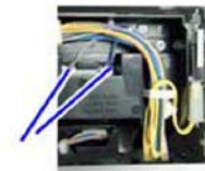
Booklet stapler move home sensor and booklet stapler move position sensor
